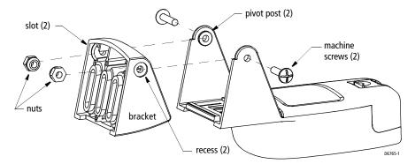
Figure 2-8: Assembling the Transducer
